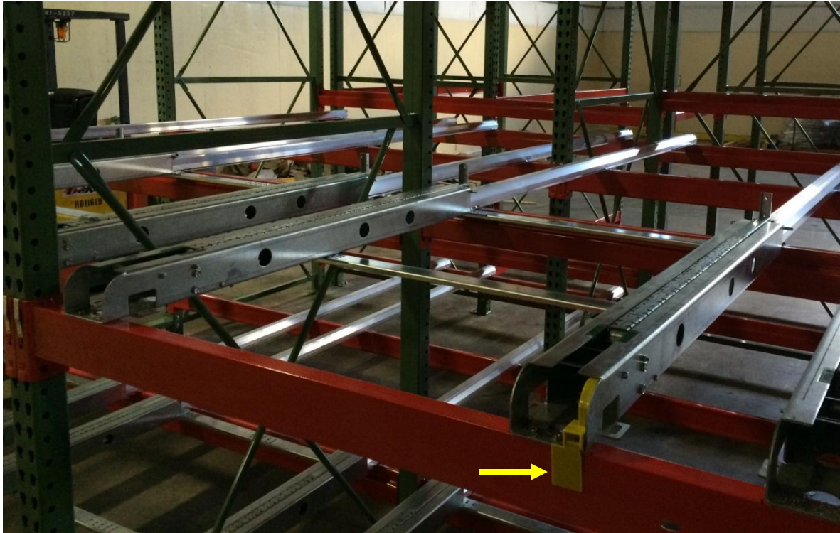
Retractable flag indicates when storage lane is full
