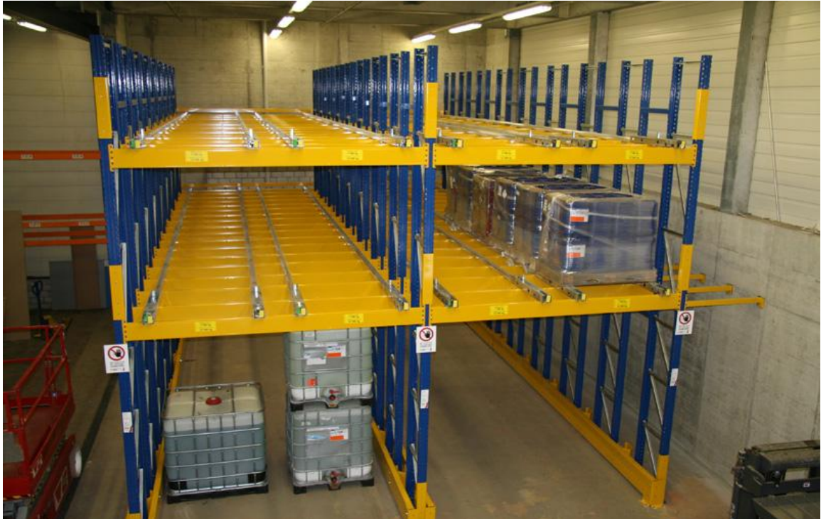
Double-stacked below, Flow-Rail above
