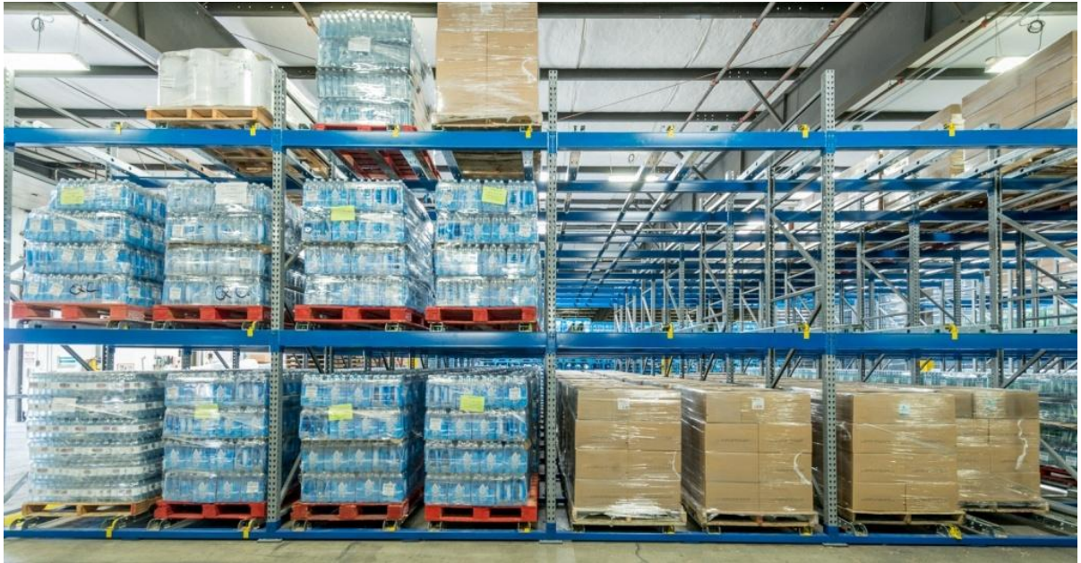
Tracks only 3.5" high optimizes vertical space
